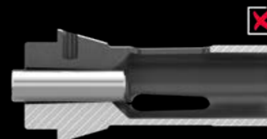
Visualization of a punctual ring clamping in the rear area of the clamping surface
