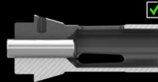
Visualization of a form-fit and cylindrical clamping
