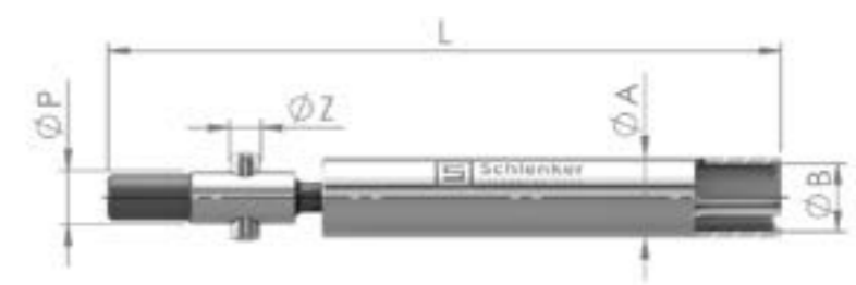
A Outside diameter B Feed rod interface P Fit ID Z Cross bore ID L Total length
